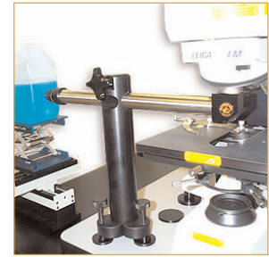
inVia Raman microscope using a custom adapter for the analysis of bulk aqueous samples
