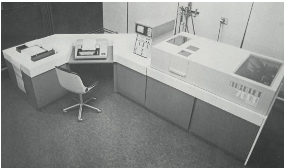
Figure 5.8. Interferometer, incorporating a separate reference interferometer for the laser and white light.
