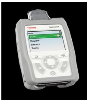
Thermo Ahura hand held First Defender – for untrained user
