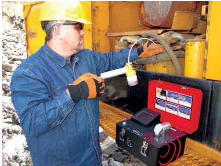
Interspectrum 9kg, 21x22 cm, ATR On the job use, dedicated analyzer
