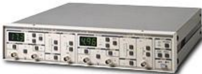
Filter: 115 dB/octave rolloff, 1 Hz to 100 kHz range
