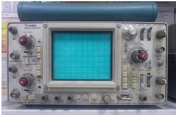
Type 465 Tektronix oscilloscope, popular analog oscilloscope, portable, and representative.
